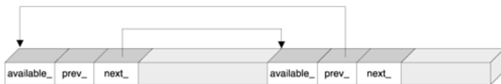
Figure 4.2. An allocator with constant-time deallocations
