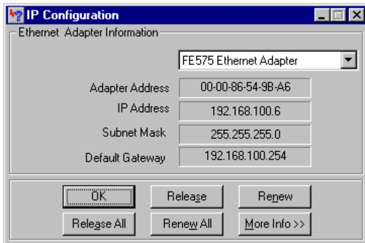
The IP address and the default gateway should be in the same network or subnet. Otherwise, this host would not be able to communicate outside the network. In the previous figure the subnet mask tells us that the first three octets must be the same to be in the same network. IP addressing will be discussed in Module 9.
