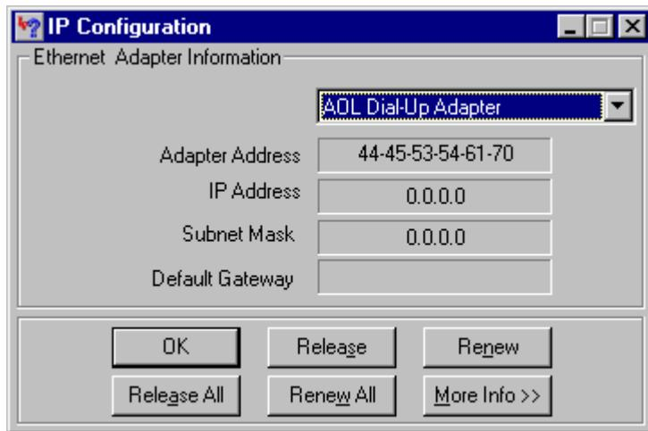
Be sure to return to the adapter that displays the NIC or modem data with an IP address
