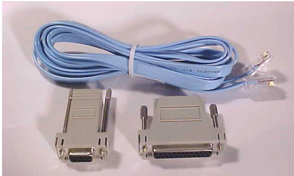
This cable is called a rollover because the pins on one end are all reversed on the other end as though one end of the cable was rotated or rolled over. In the last lab when building the straight-through cable, putting the second RJ-45 on upside down would have made a rollover cable instead of the straight through cable.
