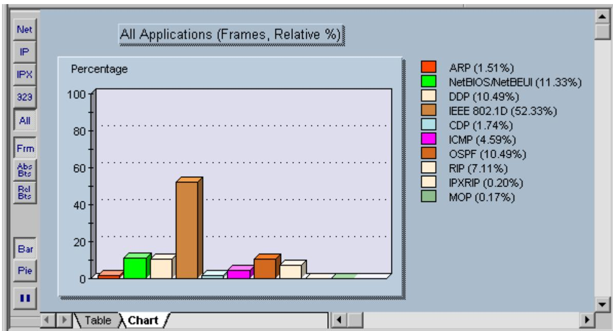
Try each of the buttons and tabs to see the results. The **Net** button shows only network protocols. The **323** button refers to the H323 Voiceover IP protocols. Depending on the version of Protocol Expert or Inspector that is being used, this button may be called VoIP. Look at the **Frm** (frame) and the **Abs Bts** (absolute bytes) and **Rel Bts** (relative bytes) to see the results. Remember that the **Pause** button stops the capture.
