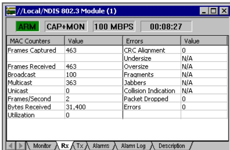
Using the console connection to the router, ping the monitoring host (192.168.1.10 or 192.168.2.10), and notice that **Unicast** frames appear. Unfortunately, the errors shown in the third column will not appear in the lab exercise unless a traffic generator like the Fluke Networks OptiView product has been added.
