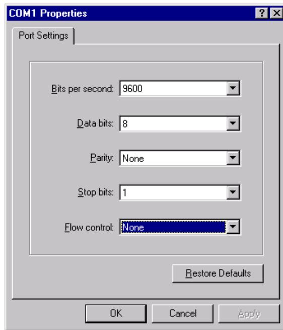
c. When the HyperTerminal session window comes up, turn on the router or if router is already on, press the **Enter** key. There should be a response from the router.
