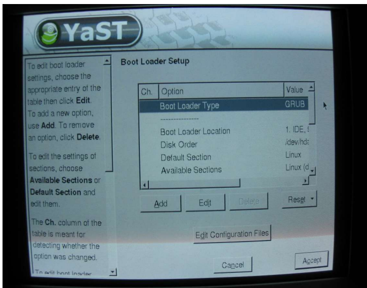
Figure 6. The Boot Loader Setup screen allows you to edit various boot loader options.
