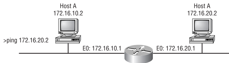
FIGURE 5.1 IP routing example using two hosts and one router
