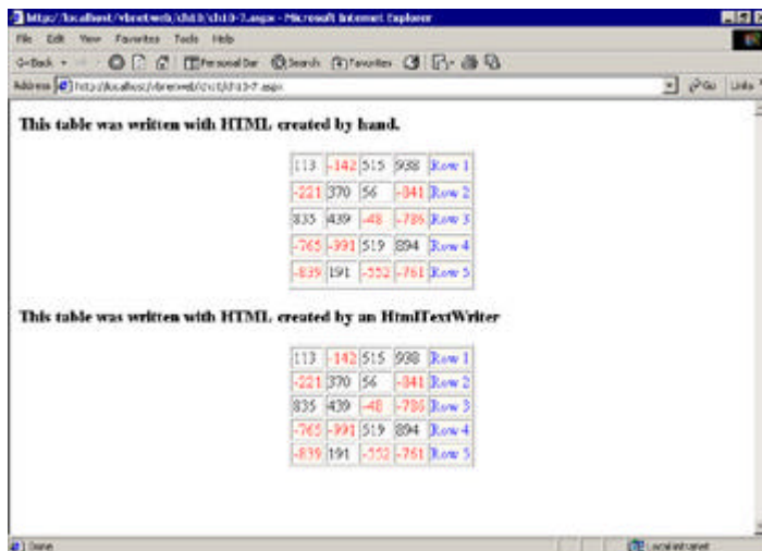
Figure 10.4: Custom HTML versus HtmlTextWriter: two table examples Listing 10.6 shows the code. The Web Form ch10-7.aspx creates some randomized data when it loads and then calls the two subroutines showTable1 and showTable2 that create the tables.
