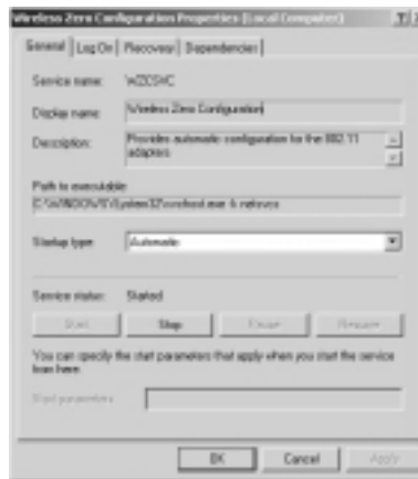
Figure 4.1 Viewing the Wireless Zero Configuration Service
