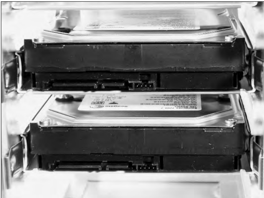
Figure 25-4: Disk drives mounted in chassis
